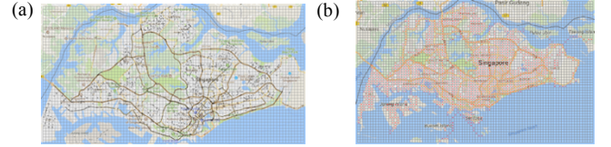
Figure 2. Singapore map overlaid with the grid map. (a) lines denote road links with installed VLDs; (b) points denote traversable grids.
